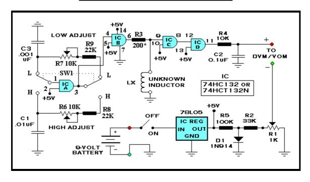
All components are 10% tolerance. 1N4146 or equivalent may be substituted for D1. An LM7805 may be substituted for the 78L05. All fixed resistors are 1/4 watt carbon composition. Capacitors are in uF. R3 value may need to be increased or decreased slightly if calibration cannot be achieved as described in text.
