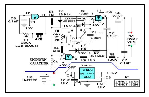
All components are 10% tolerance. An LM7805 may be substituted for the 78L05. All fixed resistors are 1/4 watt carbon composition. Capacitors are in uF unless otherwise indicated.
